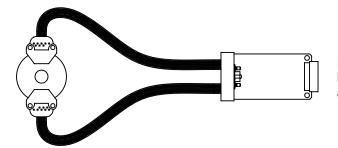
Reading two readheads on one common disc/hub assembly into one VK decoder. Good for applications where high accuracy is required.
