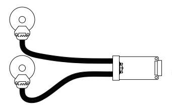
Reading two separate readheads & disc/hub assemblies into one VK decoder. Good for Az & El gimbal applications
